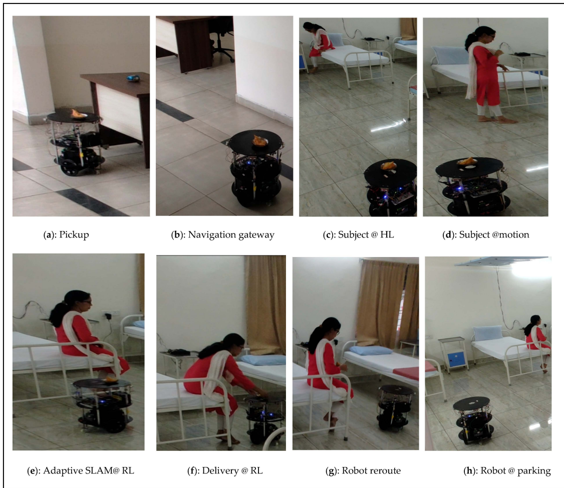
Figure 16. (a–h) Demonstration results of human and robot interaction at adaptive position.
