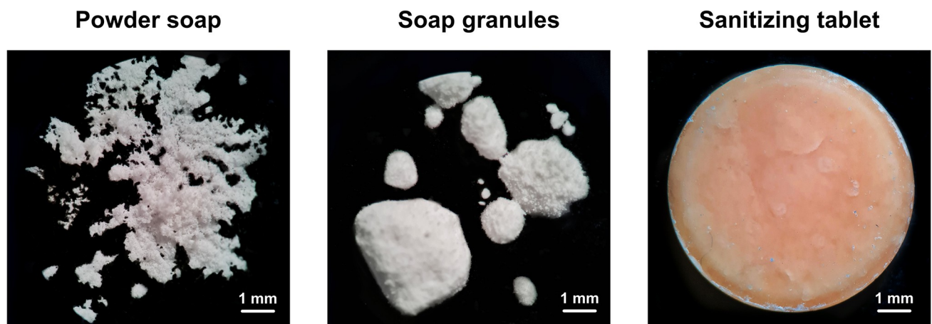
Fig 5. Optical microscopy images. Photographs obtained for the powder soap, granules, and sanitizer tablet at a 4.5 × magnification.
