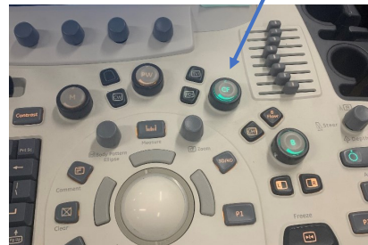
Figure 26 Twinkling and Doppler gain. Doppler GN is operator-dependent and strives to strike a balance between twinkling and noise. The maximum gain on this ultrasound scanner is 30.0. When the GN is set too low (GN =10.0), noise is filtered out but so is a substantial component of twinkling. When the GN is set too high (GN =27.0), noise can confound the twinkling signature. The GN is often selected to just below the level of noise, in this case GN =18.0, that demonstrates twinkling with very minimal, if any, noise. GN, gain; CF, color flow.
