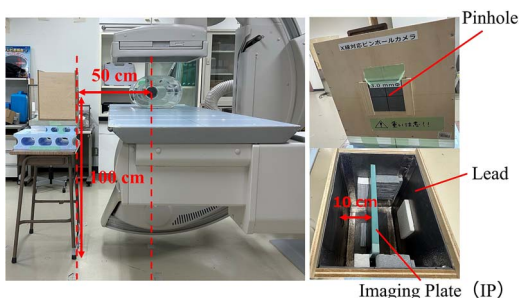
Figure 1. Layout of lead pinhole camera.
