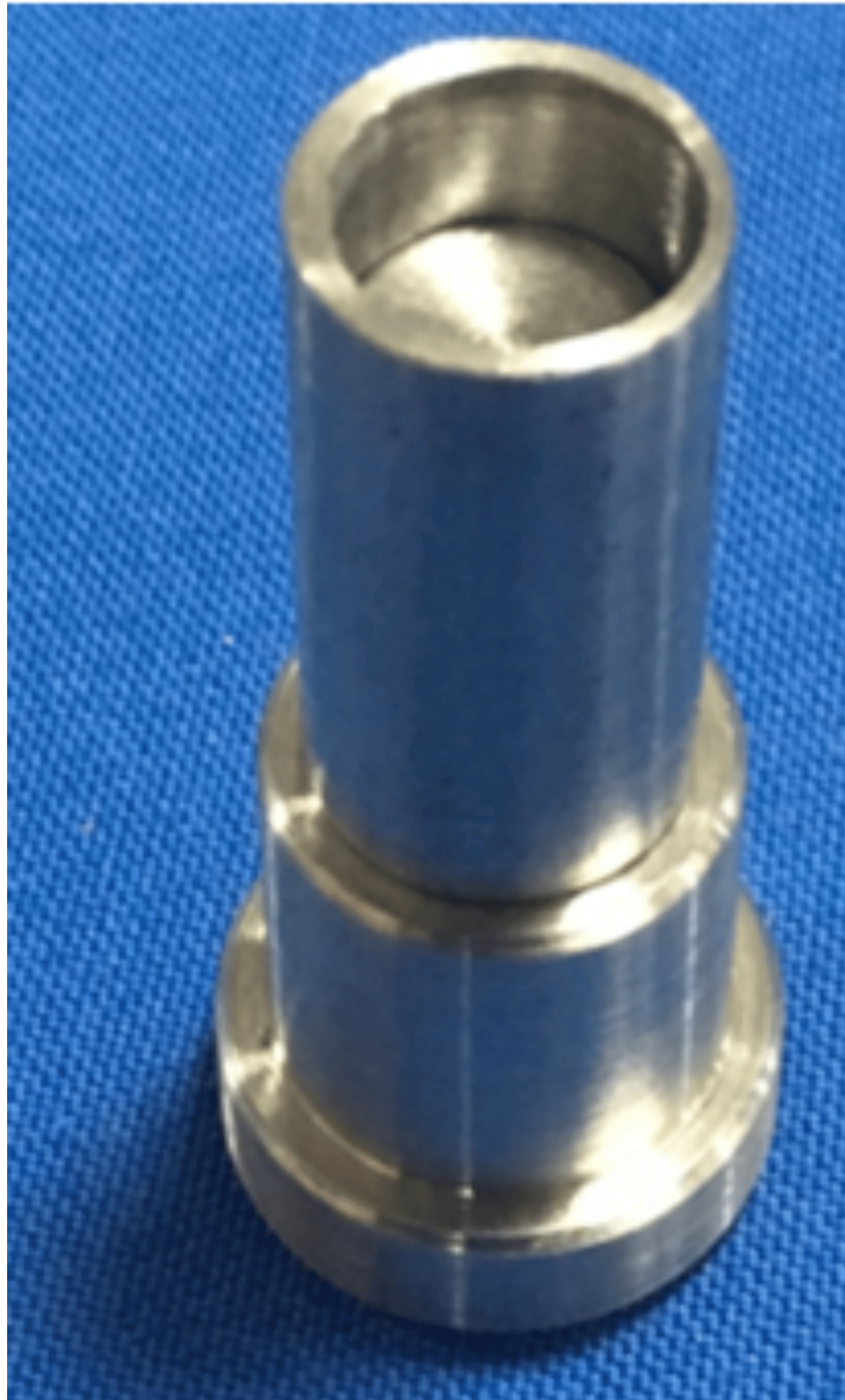
FIGURE 2: Snugly fit hollow cylindrical die over the metal jig
