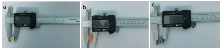
FIGURE 7: Linear dimensional change measured using a vernier caliper: (a) Ramitec, (b) O-Bite, (c) and Bona-Bite
