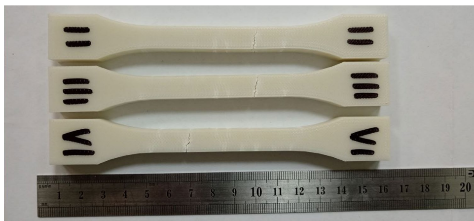
Fig. 3. Samples made by FDM printing technology from PLA plastic and subjected to tensile tests.
