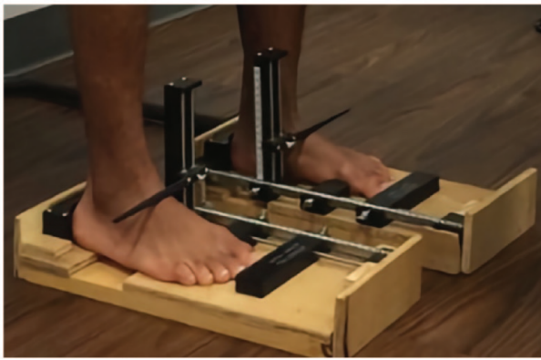
Figure 2. AHI measures were taken to classify arch type and to calculate arch rigidity and stiffness. AHI, arch height index.
