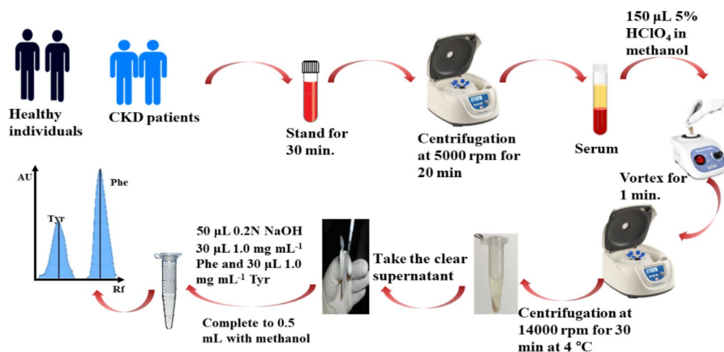
Fig. 1. Procedure for the preparation of serum samples for Phe and Tyr determination by the developed method.
