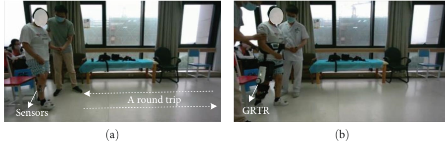
FIGURE 6: Experimental settings: (a) the test without exoskeleton and (b) the test with assistance from exoskeleton.
