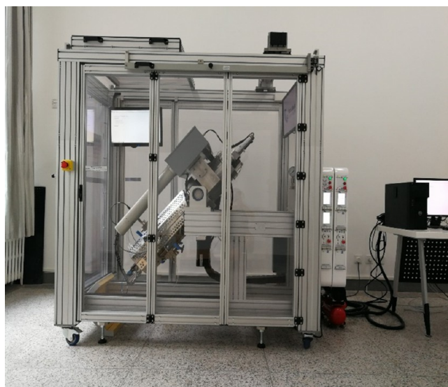
Figure 2. Ultrahigh-voltage full visual PVT testing system
