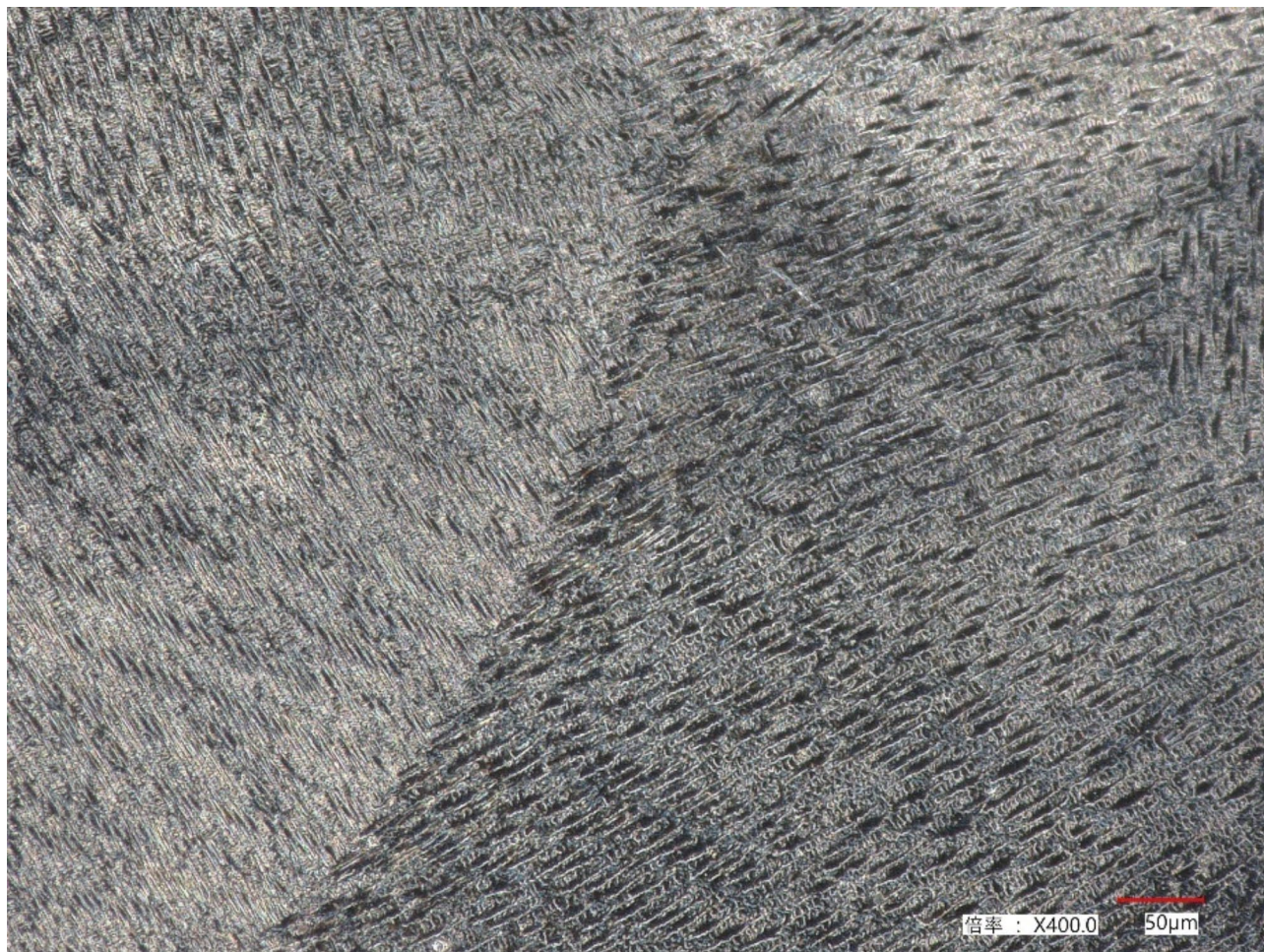
Fig. 13. Microstructure result of 25%SS316L-75%IN718.
