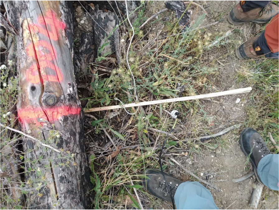
Fig. 2. measurement of soil moisture (black cable) and soil temperature (white cable) along the sampling transect. In this case, soil temperature is measured in the position “flush_downhill” (the picture is not perfectly taken from nadir), while soil moisture is measured in the position “downhill”.
