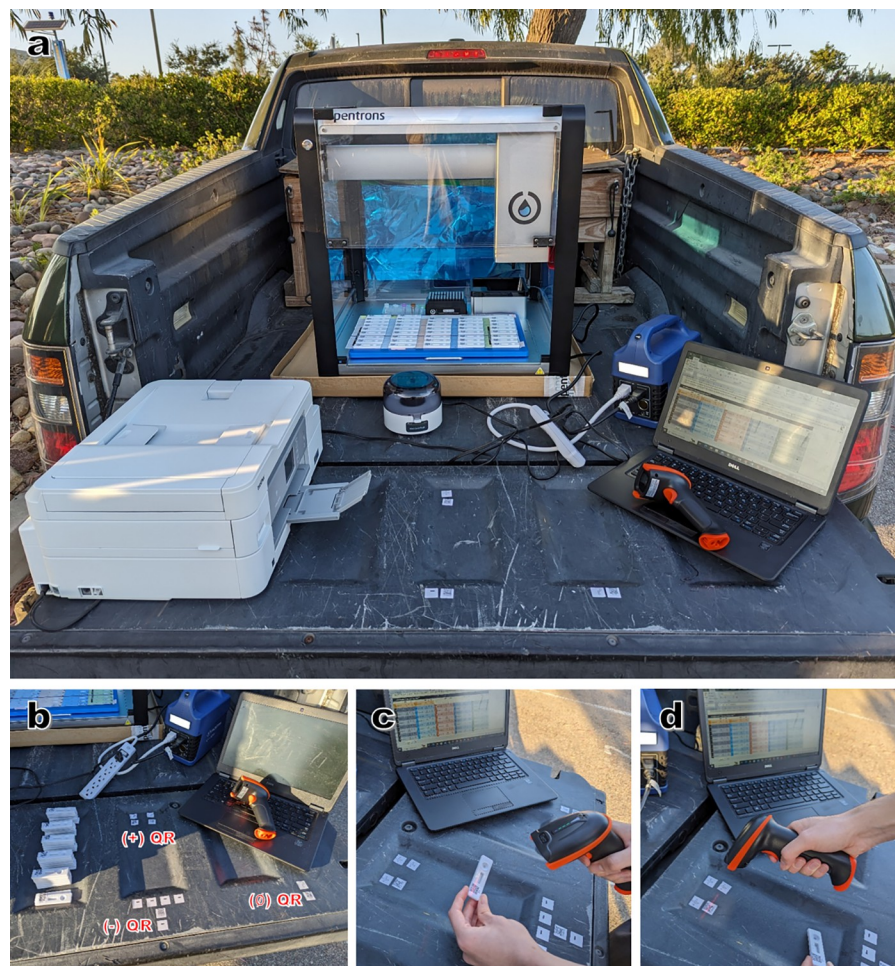
Fig 2. Embodiment of field testing station for use of rtWIZARD protocol. (a) A portable power bank can power several pieces of equipment including the OT-2, laptop computer, a centrifuge, an office printer, and lights. (b) The rtWIZARD QR code sheet includes codes for resulting by scanner. The rtWIZARD plate record spreadsheet includes (c) a script/macro for automatic cursor movement and (d) these cells can be populated by scanner as well.
