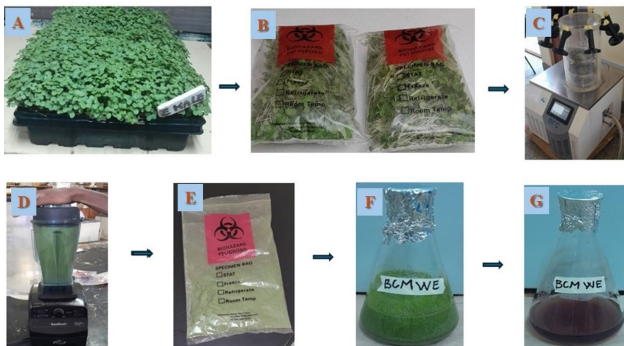
Fig. 1. An illustration of plant sample collection, drying, and extraction process. (A) Microgreens ready to be harvested, (B) The microgreens were harvested and stored in a sterile bag for transport to the lab, (C) Microgreens freeze-dried process utilizing a freeze dryer, (D) Microgreens grinding using a grinder, (E) Microgreen powder, (F) Microgreen powder soaked in water for extraction, (G) Microgreen aqueous extract.
