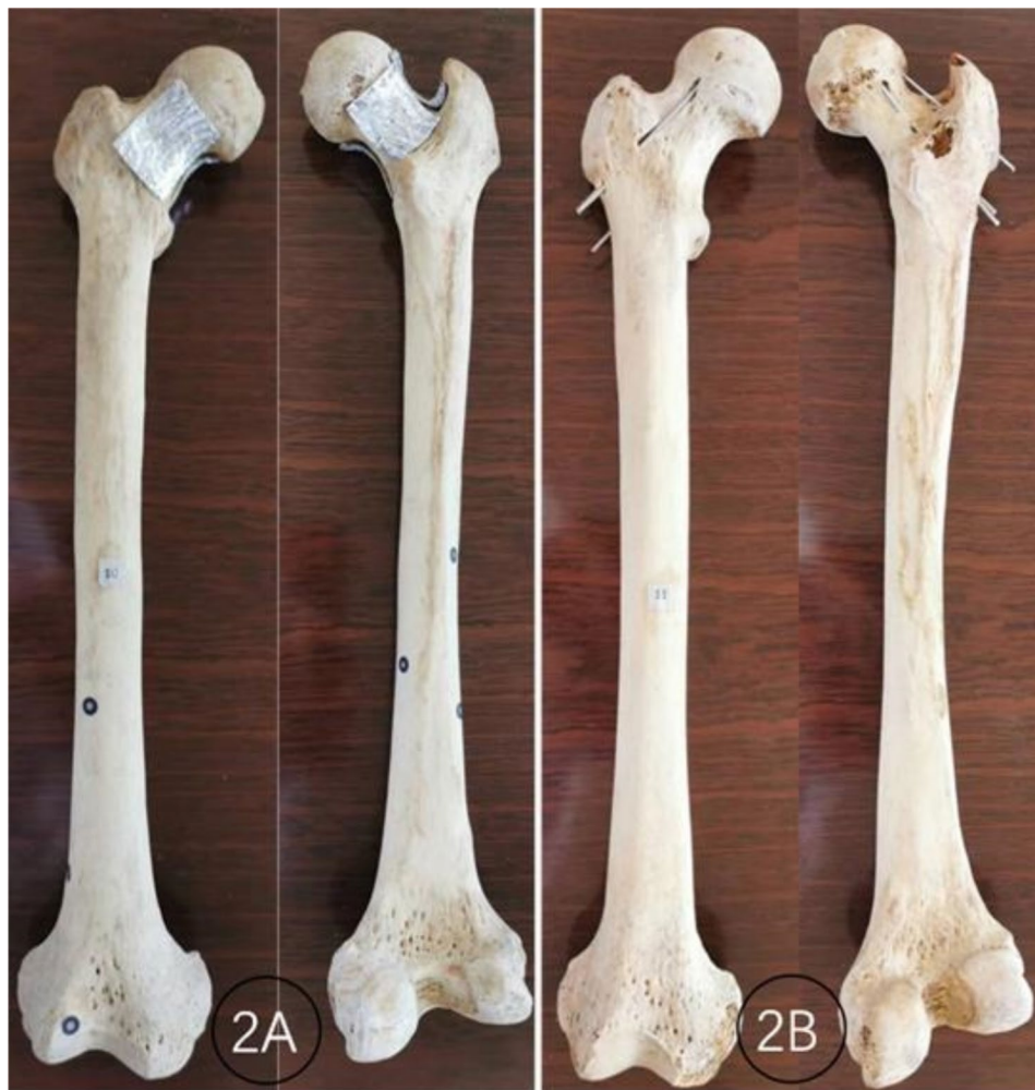
Fig. 2 Model of the femoral neck wall attached to steel wire wind aluminium foil (2 A) and a model of three Kirschner wires perforating the femoral neck wall
