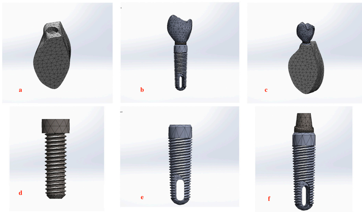
Figure 1. Meshing of structures: (a) 3D meshing of bone. (b) 3D meshing assembly of implant–abutment and crown complex. (c) 3D meshing of final model within bone. (d) 3D meshing of abutment screw. (e) 3D meshing of implant fixture. (f) 3D meshing of implant–abutment assembly.
