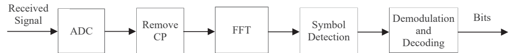
Figure 3. Processing at the receiver. The received time-domain signal is first converted into a digital signal via an ADC, followed by the removal of the cyclic prefix. After undergoing an FFT, the signal is converted to the frequency domain. In the frequency domain, it passes through the symbol detection module, as well as the demodulation and decoding module, resulting in the output information bits.
