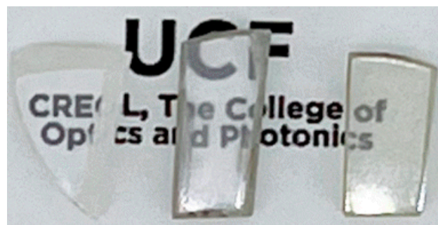
Figure 5. From left to right: untreated, annealed, and Sample #3.
