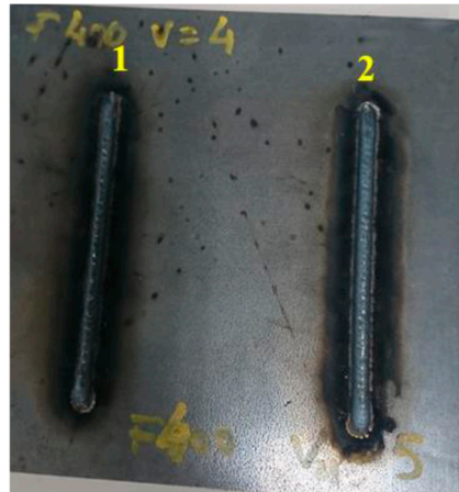
Figure 7. Test 5 (1) bead with wf = 4 m/min and ts = 400 mm/min, (2) bead with wf = 5 m/min and ts = 400 mm/min.
