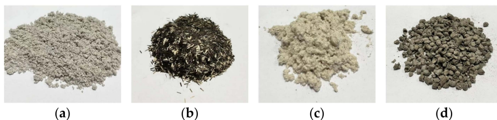
Figure 1. Morphologies of fiber additives. (a) Flocculent basalt fiber; (b) chopped basalt fiber; (c) flocculent lignin fiber; (d) granular lignin fiber.
