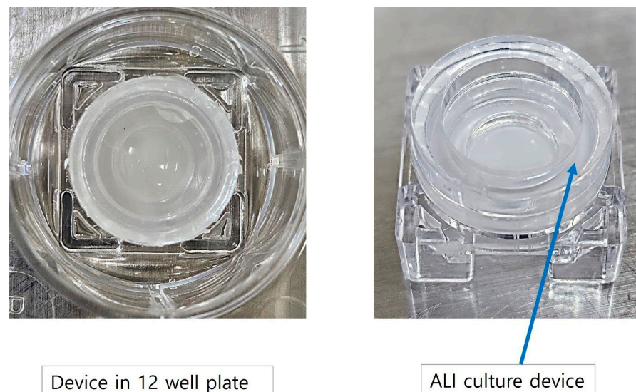
Figure 5. Respiratory mucosa-on-a-chip model in 12-well plate. The air–liquid interface culture device was placed in the 12-well plate (left) and three parts of the mucosa-on-a-chip were connected for respiratory differentiation (right).
