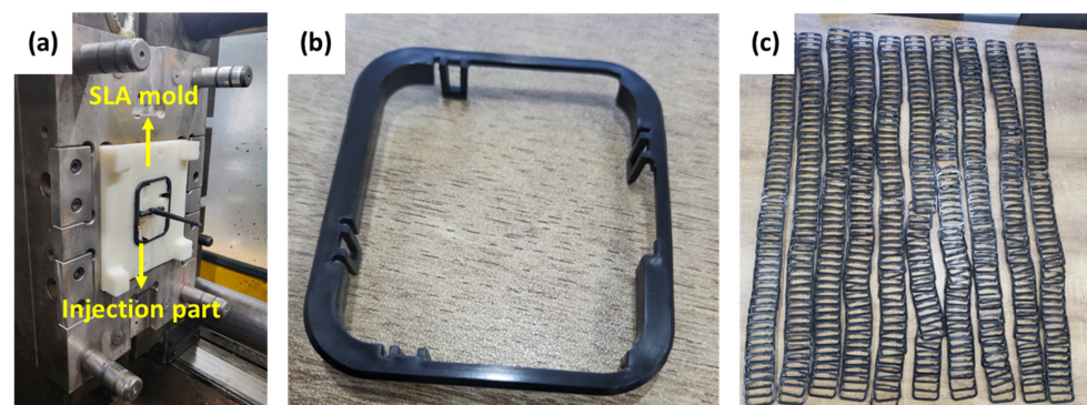
Figure 8. Photographs of the equipment of the SLA mold and injection part: (a) SLA mold; (b,c) Injection parts.
