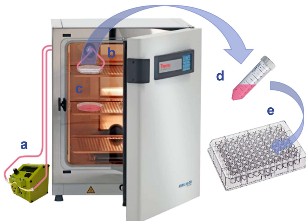
Figure 2. Diagram of the perfused-medium leaching & MTT assay. (a) Peristaltic pump. (b) MiFD with medium perfusion. (c) Control-medium. (d) Perfused medium extracted. (e) 96-well plate for the MTT assay of the perfused medium.
