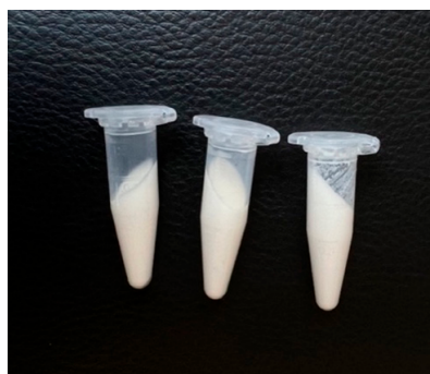
Figure 4. Bigel samples after centrifugation (from left to right: ABG1, ABG2, and ABG6).
