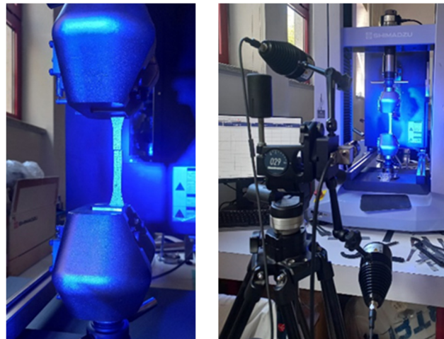
Figure 7. Tensile test and Digital Image Correlation setup.
