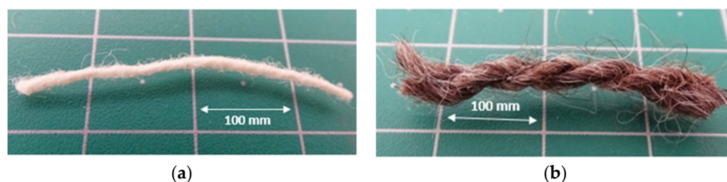
Figure 1. Yarns of the fibres used on the composites—(a) Sheep's wool yarn; (b) Dog wool yarn.
