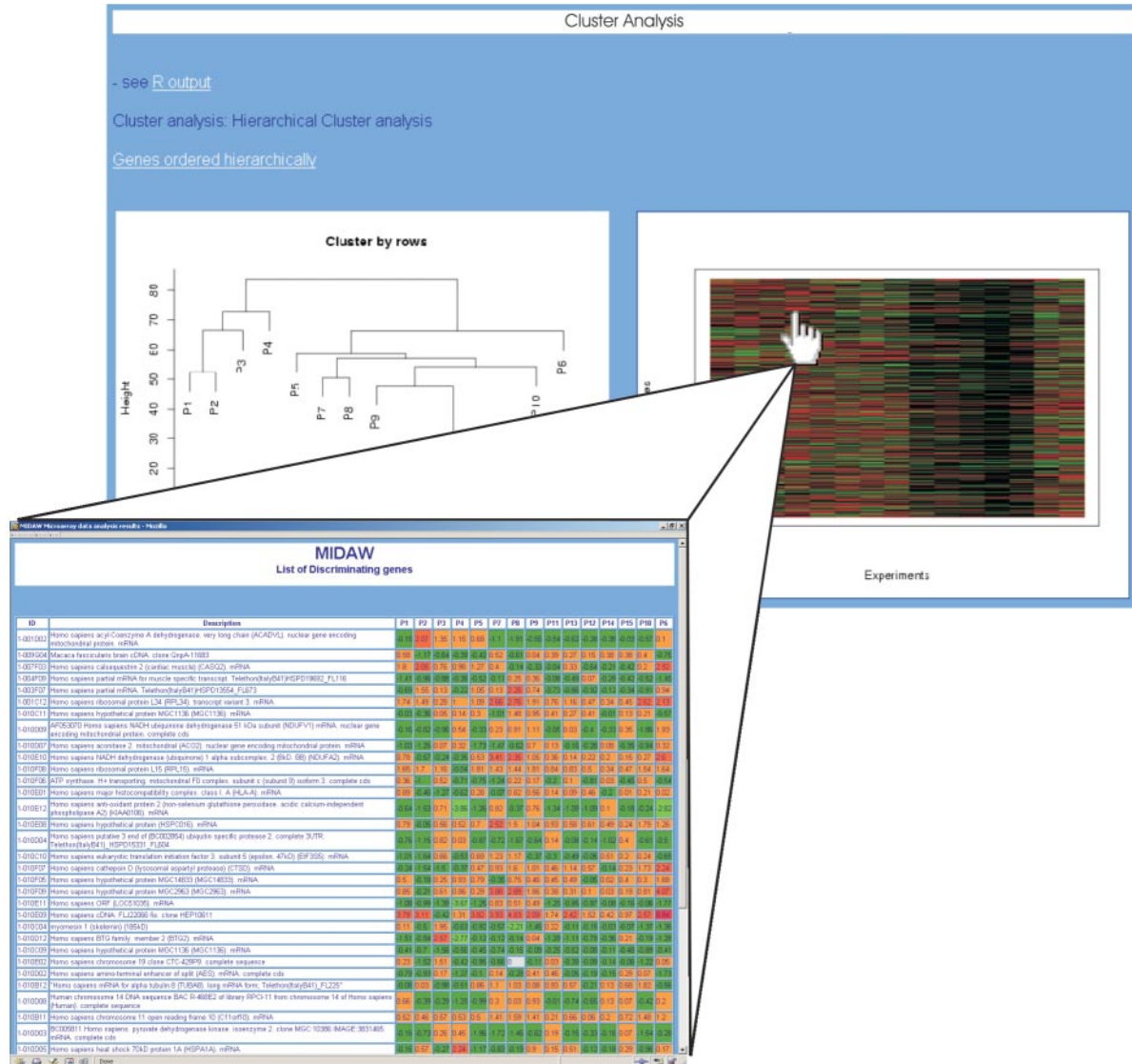
Figure 3. Zoom section of the cluster analysis step. The image of expression profiles is an HTML map that shows a table with descriptions and expression values of the genes that lie in a specific area selected by the user.
