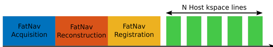
FIGURE 1 Schematic of product GRE sequence with FatNav navigator embedded every N host k -space lines.
