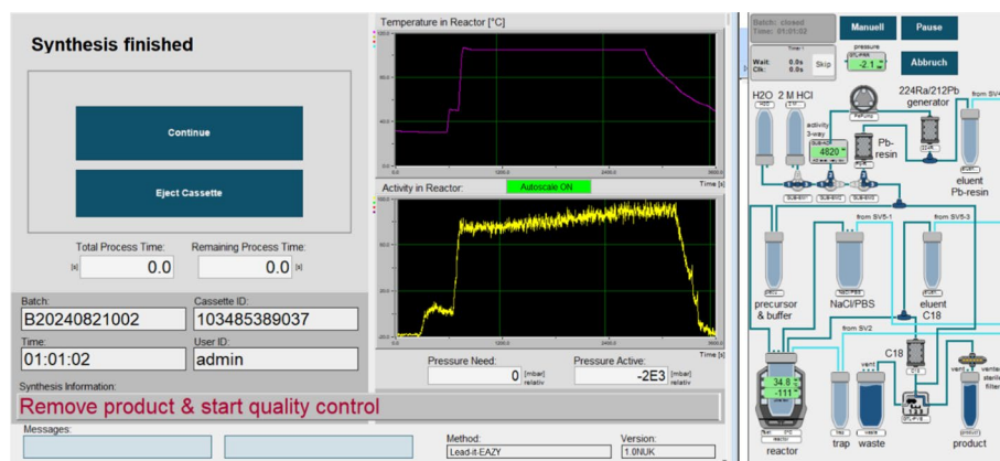
Fig. 2 Schematic depiction and typical graphs for activity level and temperature of the Lead-it-EAZY process on the ML EAZY module
