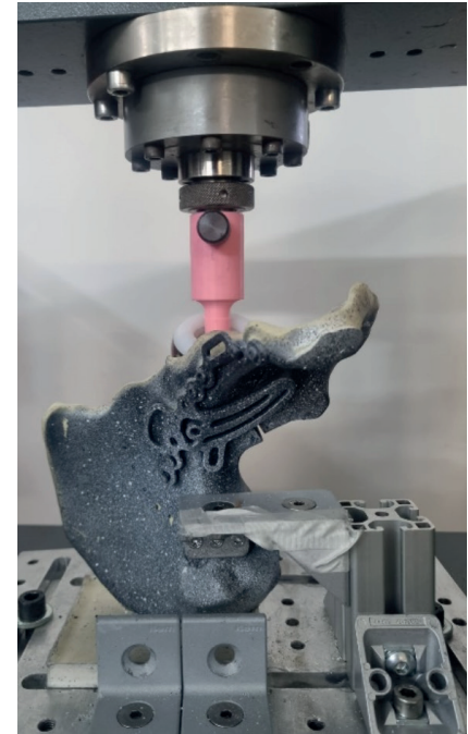
Figure 2. Force was applied in a medio-superior direction through the hemiarthroplasty using a previously described test set-up [20-24].
