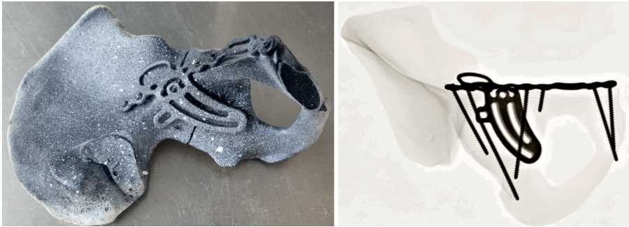
Figure 1. A T-shaped acetabular fracture was fixed with a biplanar 10-hole 2-column plate osteosynthesis using either conventional screws or angular stable screws. On the left is a specimen after anatomic repositioning and fixed plate osteosynthesis. The specimens were sprayed for optical motion tracking. On the right the corresponding radiograph is displayed.
