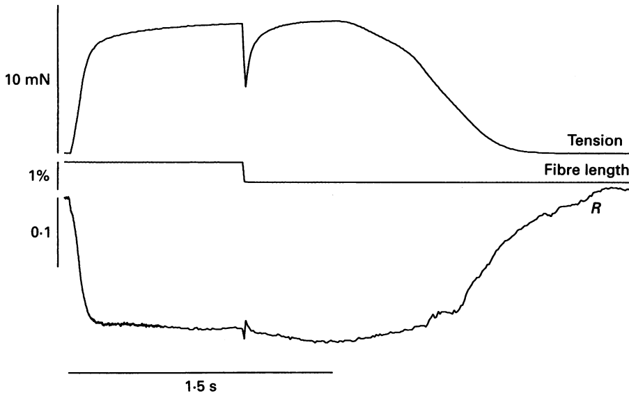
Fig. 8. Changes in tension (top), fibre length (centre) and intensity ratio R (bottom) associated with a 1.5 s tetanus at resting sarcomere length 2.55 \mu\text{m} ; fibre slightly compressed between glass plates. A release of 0.92% fibre length, complete in 0.2 ms, was imposed at 1 s in the tetanus. Peak retardation at the thickest part of fibre cross-section ( \phi_c ) before compression, 2.85 rad; after compression, 2.59 rad. The compensator retardation ( \theta ) was set to the latter value before the start of the trace. Fibre length at 2.55 \mu\text{m} sarcomere length, 7.3 mm; width, 143 \mu\text{m} ; depth, not measured. Sample interval was 1 ms for the first 550 ms and 10 ms thereafter. The latter is inadequate to resolve the changes associated with the length step; these are shown with a faster sampling rate in Fig. 9. The horizontal bar marks the stimulus.
