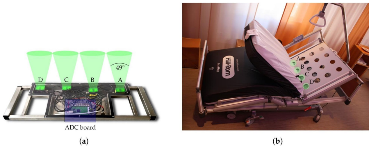
Fig. 1 (a) Radar system with four continuous-wave radar modules and ADC (Analog to Digital Converters) board. (b) Position of the radar modules underneath the head section of the slatted frame (indicated in green). Source: Schellenberger et al. 2020 [11]
