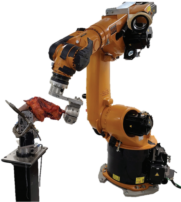
Figure 2. Experimental setup of a right shoulder with a 6 degrees of freedom robotic arm (posterior view).
