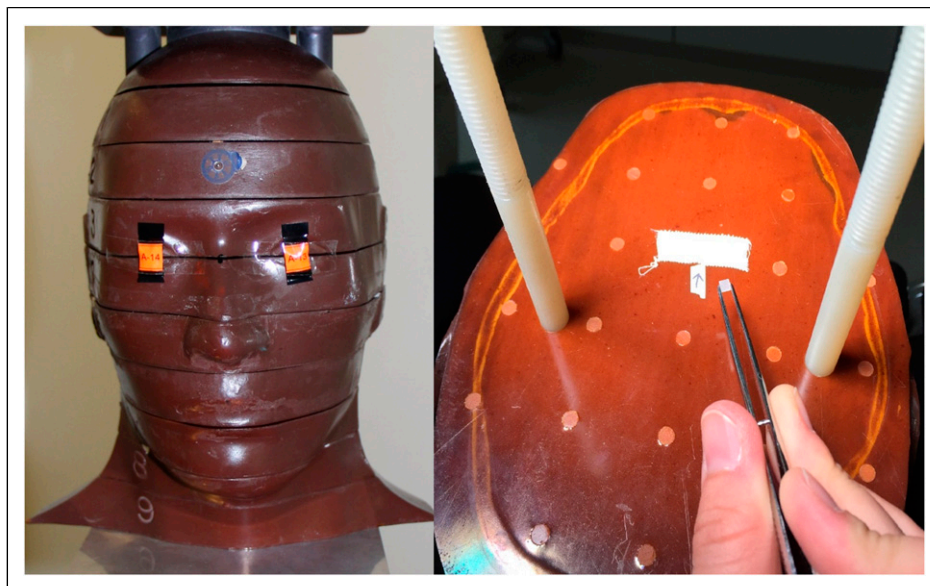
Figure 1. Image of the Alderson-Rando phantom head, location of the TLDs in the nine different axial planes.
