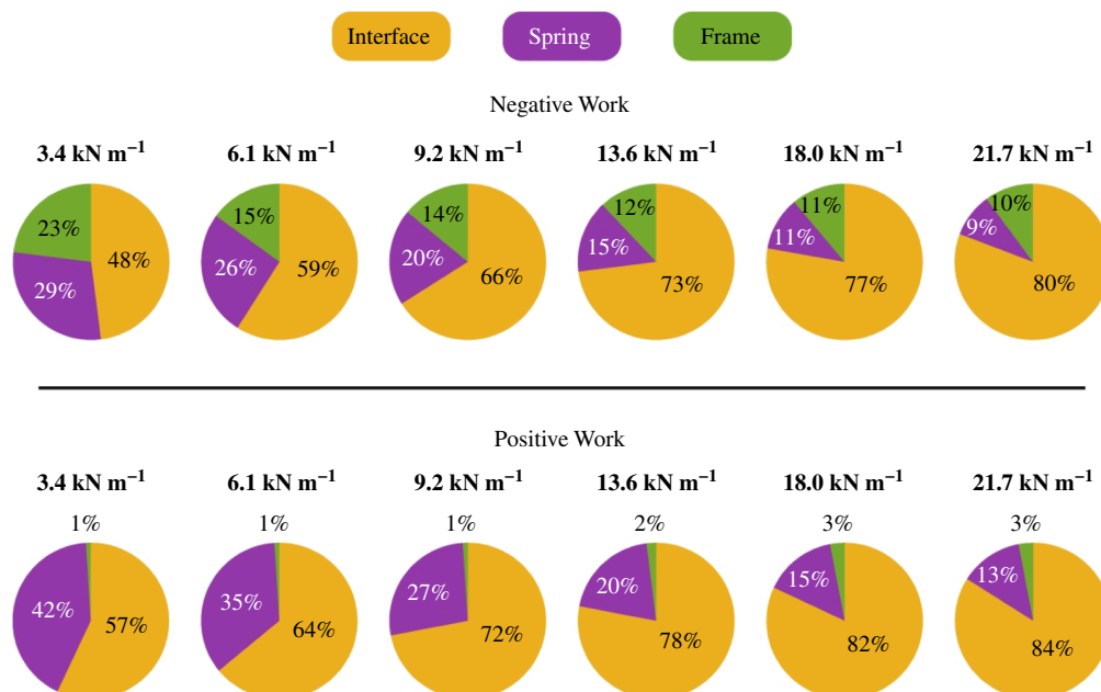
Figure 11. Relative work contributions. Pie charts show the relative contributions of the interface, spring and framework to the total negative and positive knee work. Interface work increased positive and negative work contributions relative to the other components as spring stiffness increased.
