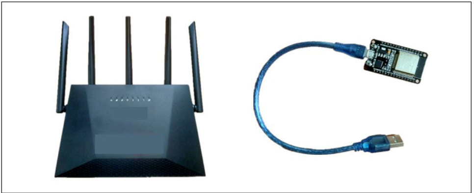
Fig. 4. Transmitter D-link AX3000 router and receiver ESP32 microcontroller.
