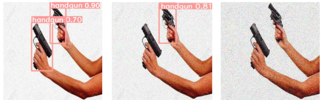
Figure 4 Effect of salt-and-pepper noise on the same test image containing two handguns: (left) 0.01-level, (center) 0.02-level and (right) 0.05-level. (Note: The original image within this figure can be found in the DaSCI Weapon Detection dataset, and it is distributed under the terms of the Creative Commons Attribution 4.0 International).
