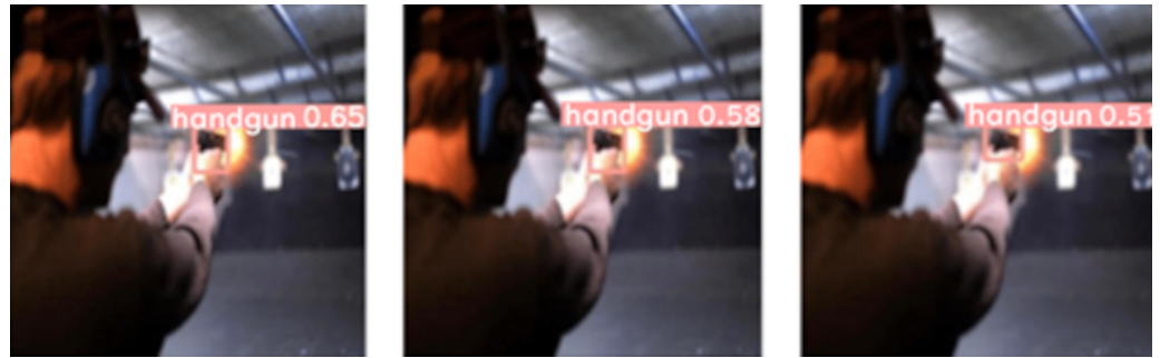
Figure 6 Effect of Gaussian blur using tested kernel sizes k on the same test image: (left) k = 3 , (center) k = 9 and (right) k = 13 . (Note: The original image within this figure can be found in the DaSCI Weapon Detection dataset, and it is distributed under the terms of the Creative Commons Attribution 4.0 International).
