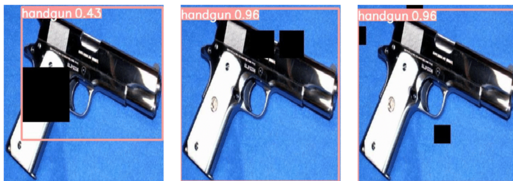
Figure 5 Effect of synthetic random occlusions on the same test image: (left) one occlusion of 30% image size, (center) two occlusions of 15% and (right) three occlusions of 30%. (Note: The original image within this figure can be found in the DaSCI Weapon Detection dataset, and it is distributed under the terms of the Creative Commons Attribution 4.0 International).
