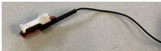
Fig. 14. contact microphone completed with 3D printed attachment.
