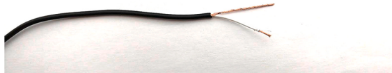
Fig. 12. Exposed end of the contact microphone wire after separating the inner and outer conductors.
