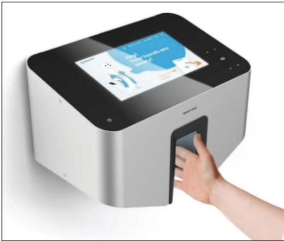
Figure 1 - Device used to record the distribution of the UV marker on the investigated surface.
