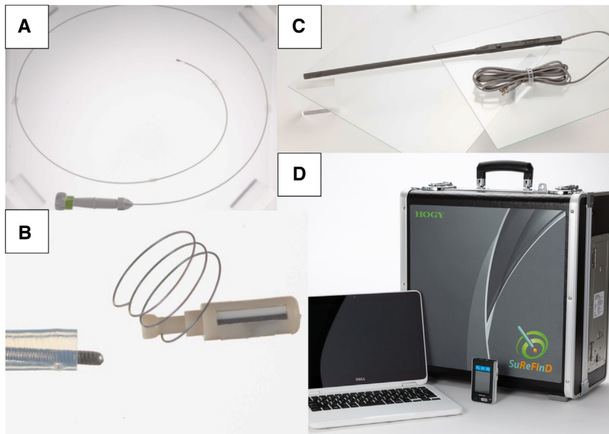
FIGURE 1. Components of the RFID lung marking system. A, Delivery device that is used through a bronchoscope with a 2-mm working channel. B, Passive RFID tag with nitinol coil (13.56 MHz; 3.2 × 1.6 × 0.9 mm). C, Detection probe (diameter, 10 mm) with 30-mm communication range. D, Signal-processing unit.
