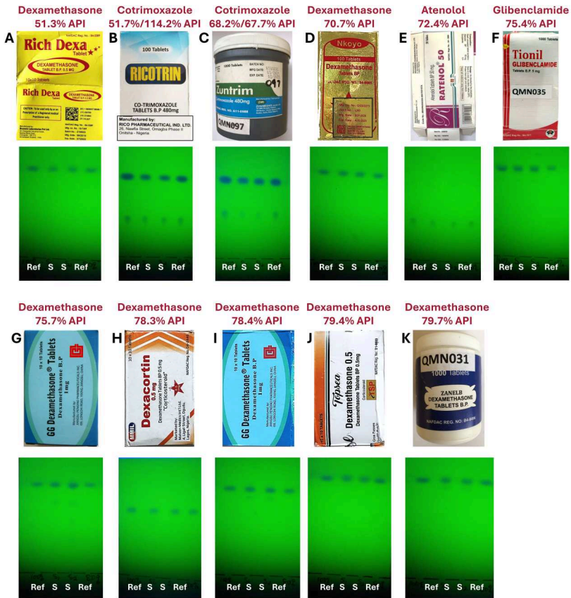
Figure 3. Thin-layer chromatographic analysis of medicines which contain between 50% and 80% of the declared amount of the active pharmaceutical ingredient.
