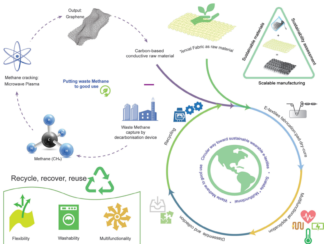
Figure 1. A comprehensive exploration of EoL options for wearable e-textiles. The process involves repurposing waste methane-derived graphene through scalable manufacturing, incorporating multifunctional applications, disassembling electrical components from textile electrodes, and analyzing EoL options. The sequence includes heat treatment by pyrolysis and mechanical recycling methods.
