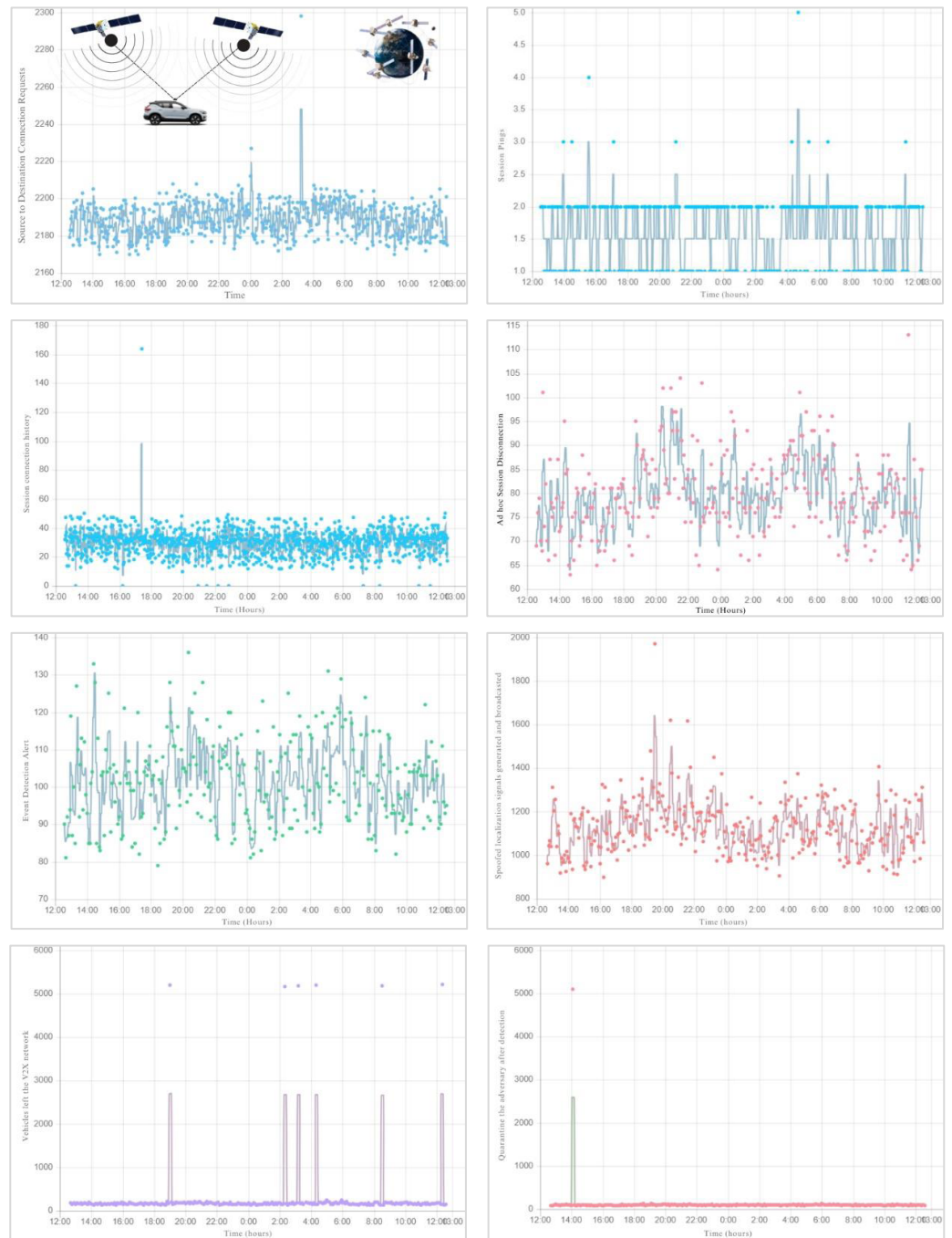
Figure 2 Emulation processes in the controlled environment. (A) The chart tracks the number of source to destination connection requests over a 24-hour period, depicted as a scatter plot with light blue dots. These dots show fluctuations in the number of requests, ranging from approximately 2,160 to 2,300, with a noticeable spike around 2:00 AM, where the requests briefly surge. The overall pattern is dense, indicating a consistent level of activity throughout the day, with only a few significant variations in the connection requests. (continued on next page...)
