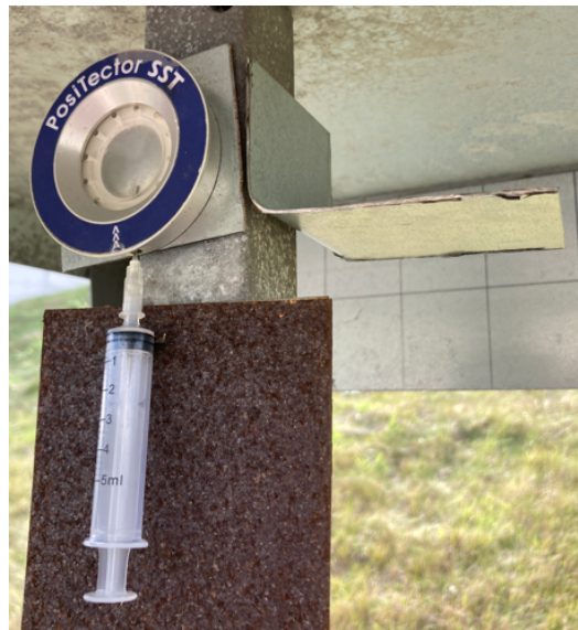
Figure 7. In situ measurement performed on a short-term coupon.
