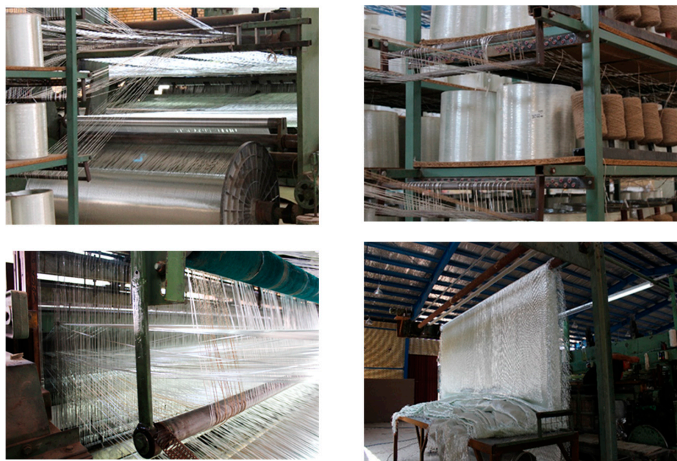
Figure 2. Images of the weaving machine producing 3D woven fabric at Novavaran Sanat Silk Co., Ltd., Kashan, Iran.
