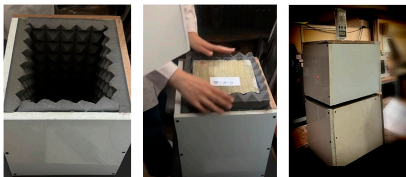
Figure 6. View of the sound measuring device (a chamber to act as an obstacle to sound transmission) in the laboratory.
