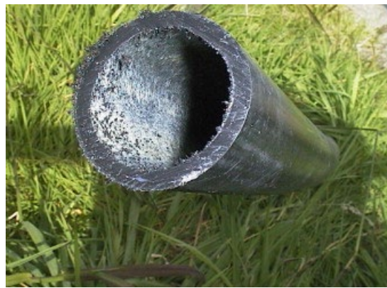
Figure 3. Concrete pipe from a geothermal power plant with an adherent biofilm of sulfur-oxidizing bacteria (white). The Wairakei Power Station is the only geothermal plant in the world with once-through cooling. Shortly after the commissioning of the plant, it was discovered that headspaces in the culverts were suffering from severe acid attacks due to the presence of the oxidation product of H 2 S, i.e., H 2 SO 4 . The pH of the surface moisture was found to be <2, which is common in the presence of “sulfur-oxidizing bacteria” that oxidizes H 2 S to sulfuric acid. Reproduced with permission from Brown and Bacon [25]. © 2008 Elsevier Ltd., Amsterdam, The Netherlands.
