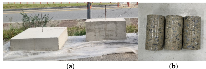
Figure 4. Specimens for mock-up test and core samples for testing: (a) slab and beam; and (b) coring specimens.
