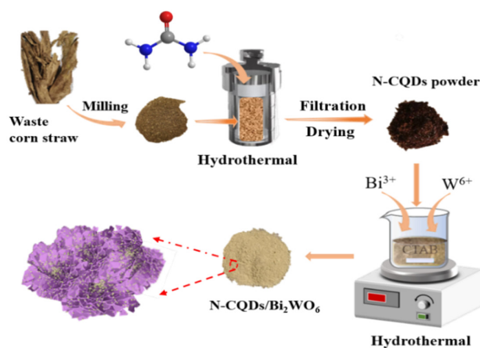
Scheme 1. Schematic description of the synthesis of N-CQDs and N-CQDs/ \text{Bi}_2\text{WO}_6 .
