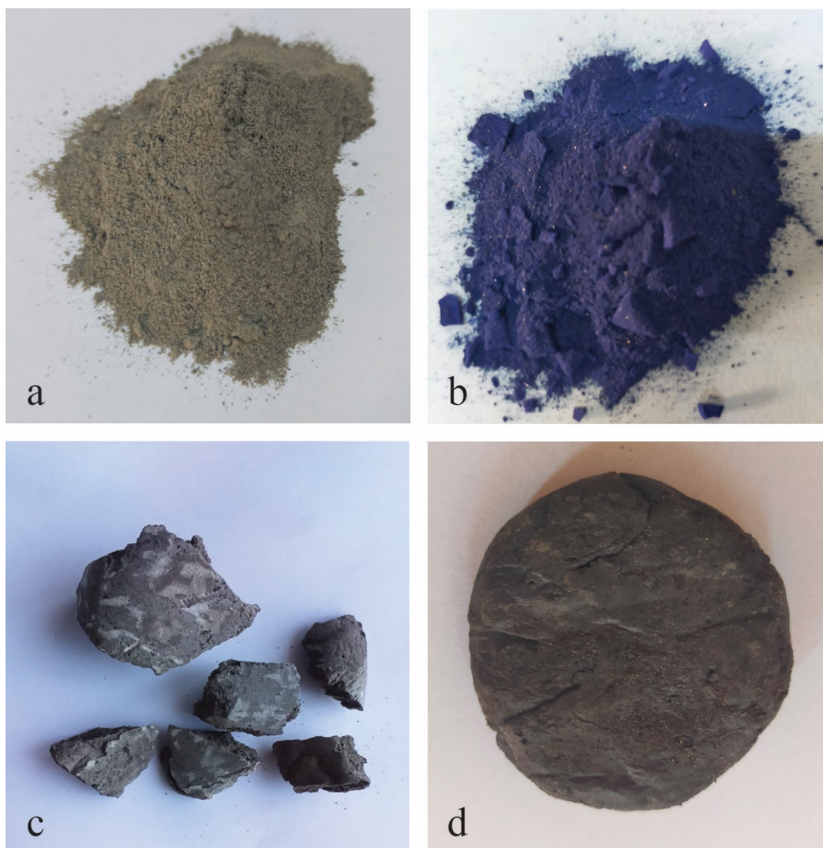
Figure 2. Stone dust (a), stone dust after CV adsorption (b), example of the S2 synthetic aggregates (c), example of synthetic aggregates with CV-embedded stone dust (d).
