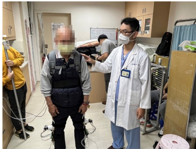
Figure 10. Clinical trials on standing balance recovery for PD patients with proposed exoskeleton robot.
