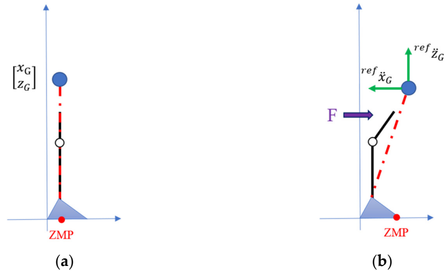
Figure 3. (a) Initial standing posture; (b) ZMP-based hip strategy for balance recovery.
