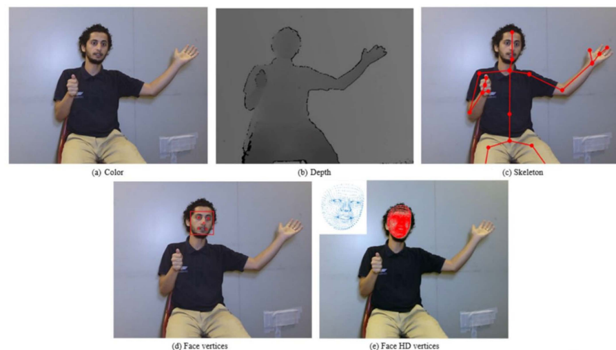
Figure 13. The mArSL dataset, an example of the five modalities provided for each sign sample [88].
